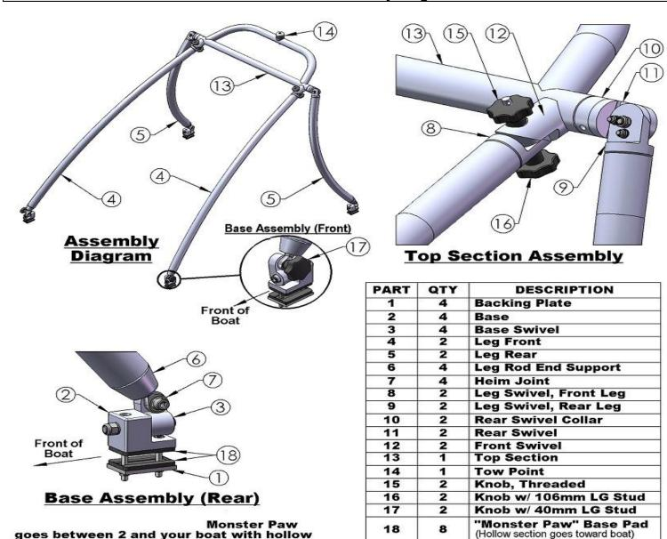
The MT2 is an innovative design in the Wakeboard Tower market that uses many common parts and design elements that make it affordable and easy to install. There are three main components of the design as shown in the <u>Assembly Diagram</u>: front legs, rear legs and the top section. The front legs are identical, and the rear legs are identical.
