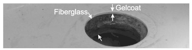
The gelcoat is a very thin layer approximately 1/16<sup>th</sup>" thick and the fiberglass below it is normally about 3/8" thick. IMPORTANT: If the fiberglass below the gelcoat is less than 3/8" thick, you need to add fiberglass cloth and/or marine treated plywood to build up the largest area available to at least 3/8" thick. You need to check all mounting points as the fiberglass thickness may vary on the boat.
